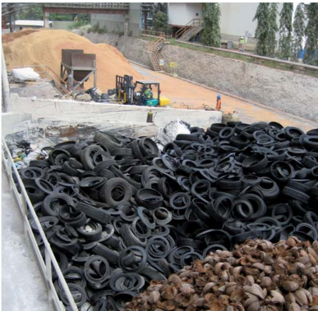
Figure 2: Coconut shells, tyres, wood chips and rice husks are used as alternative fuels in cement works
