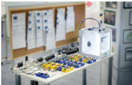
Networked with 3D printer: Arduino boards with sensors for measuring light, temperature and movement in the ROI IoT Fab
