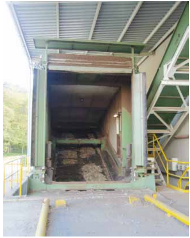
Figure 1. Unloading station with vehicle steering device. Manufacturer: Schenck Process Group T/A Redler, UK. (Source: MVW Lechtenberg).
