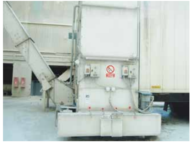
Figure 4. Mobile docking station and walking floor truck. Manufacturer: Schenck Process GmbH, Germany). (Source: MVW Lechtenberg).
