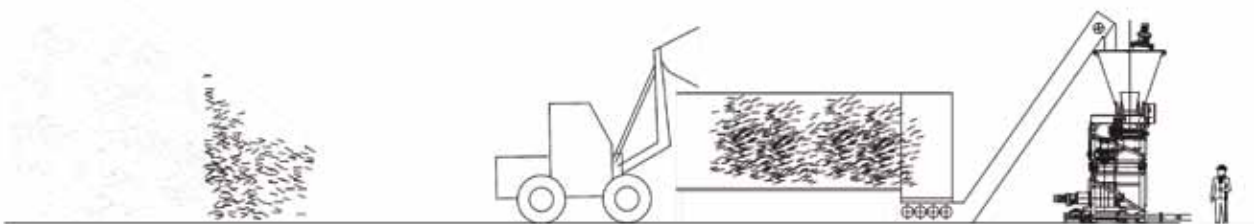
Figure 3. Open storage and wheel-loader feeding. (Source: FLSmidth Pfister GmbH, Germany).
