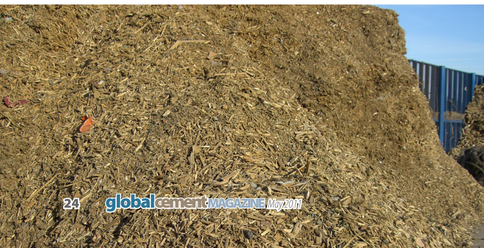
Below: Woodchips can be as an alternative fuel for cement and lime kilns.
