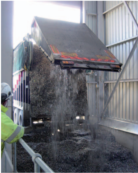
Above: Refuse-derived fuel being delivered to Lagan Cement's alternative fuels reception area.
